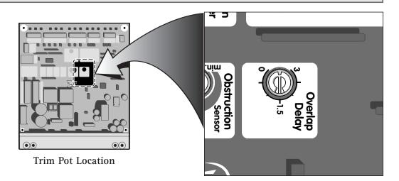
Setting the Overlap Delay Pot to any value other than zero will cause the master unit to delay in opening.
