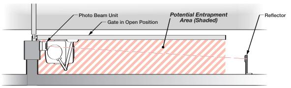
One or more non-contact sensors shall be located where the risk of entrapment or obstruction exists, such as the perimeter reachable by a moving gate or barrier.
