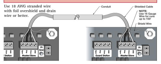
The control board provides a connector for master/slave connectivity. This connector will allow synchronized operation with a second gate operator.
