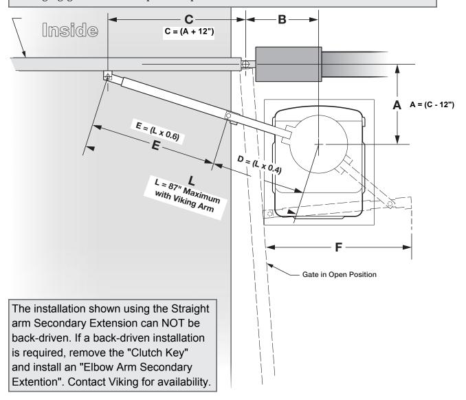
\*Note: The dimensions provided are just a guideline. Each site may have different geometries or possibilities of installation. The key for installation is to have "E" longer than "D" and to adjust the arms such that the arm is straight at the closed position.
