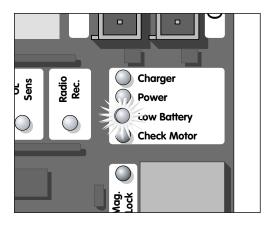
Once you put the "jumper" on the control board the "Check Motor" light will come on indicating that the Auto-Open feature has been enabled.
